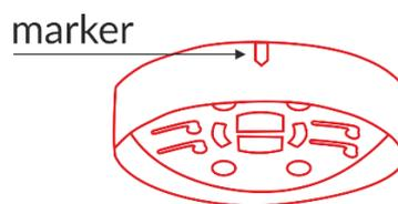
3. Fasten part 1 on the cable tray with 2-4 self-tapping screws with dimension of  $\phi 4 \times 10$ .
