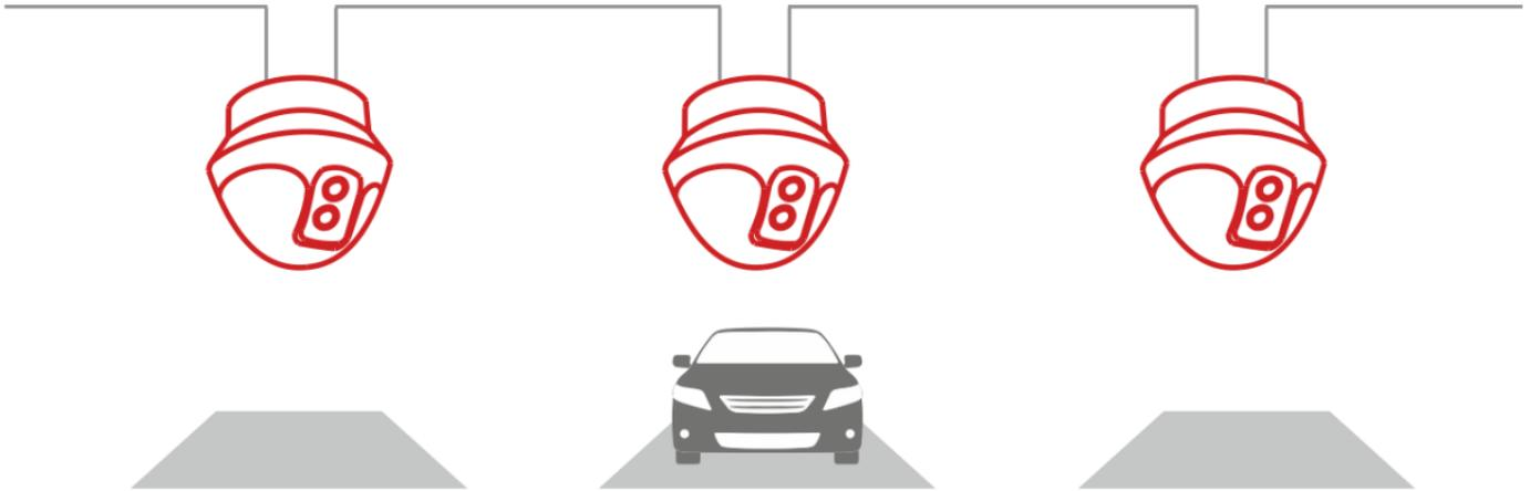
To reduce the occurrence of incorrect states, sensor should be positioned centrally to the parking space:
