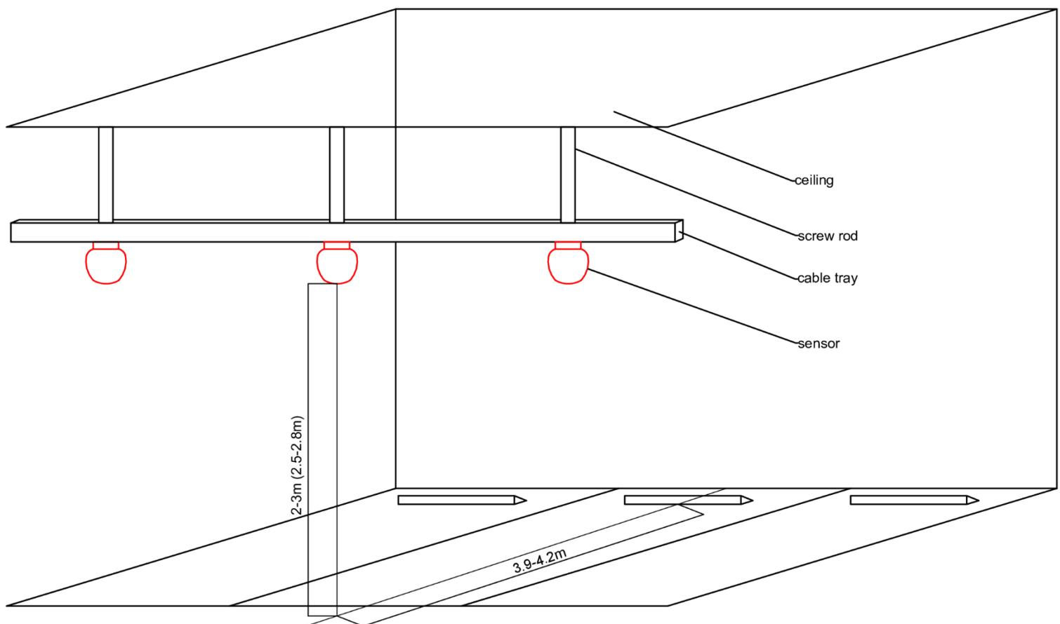
Connection of subsequent sensors in one line with approximately 3m patchcords above the parking spaces:
