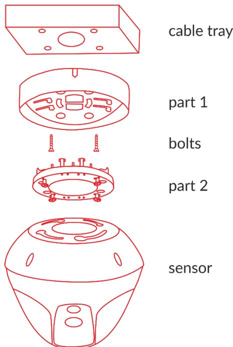
1. Cut a hole with a diameter of 40mm in the cable tray.
