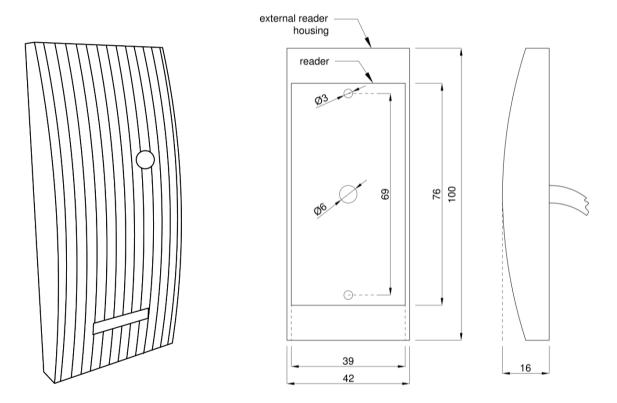
Device consists of a printed circuit board with microprocessors, signaling diodes, antenna connectors, a beeper and a dedicated antenna. In the case of external assembly, it is possible to adapt reader to work in adverse weather conditions.
