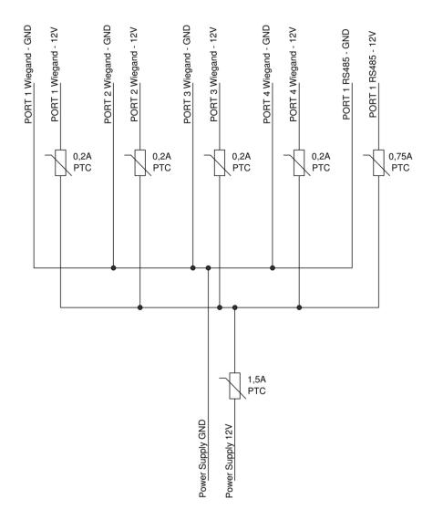
Note that the DEC relay output is located behind the 1.5A PTC fuse and it is necessary to calculate the total current consumption of the devices before connecting additional external devices to it. Exceeding the rating may lead to tripping of the fuse.
