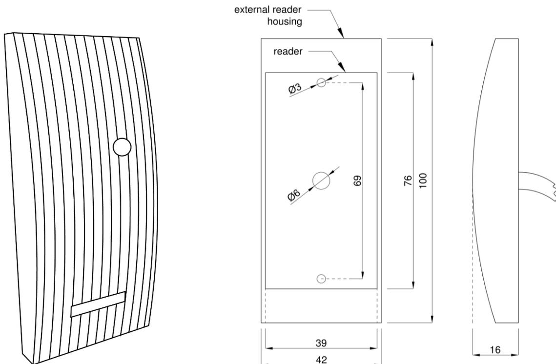
Device consists of a printed circuit board with microprocessors, signaling diodes, antenna connectors, a beeper and a dedicated antenna. In the case of external assembly, it is possible to adapt reader to work in adverse weather conditions.
